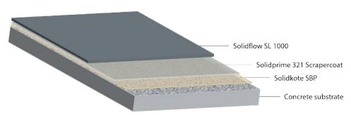
Note: The substrate should be dry to 75% RH (BS8204) and free from rising damp or ground water pressure. Damp floors should primed with **Solidkote STP Primer**.
